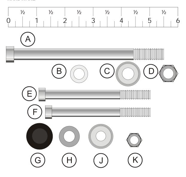
Hardware Figure 1. Assembly Parts.
